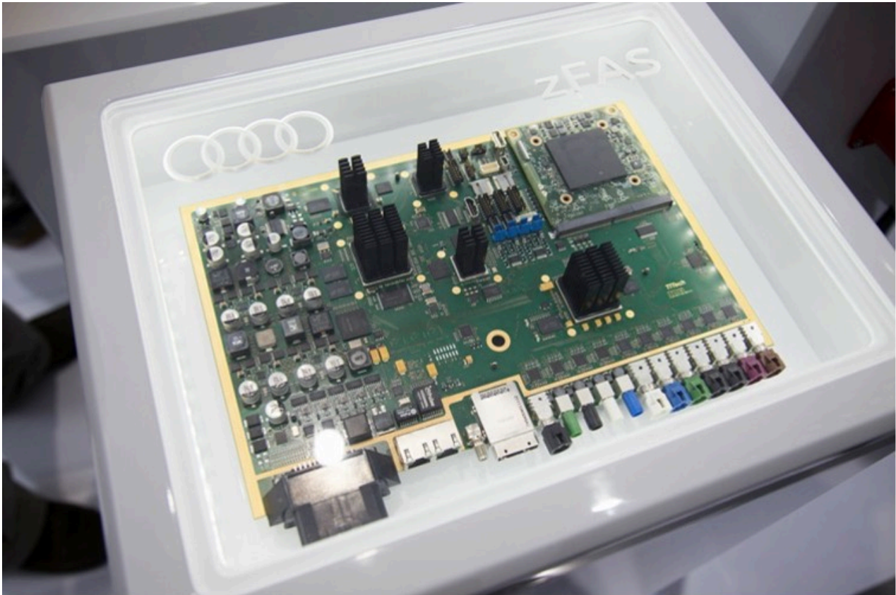
Figure 34: ADAS domain controller ECU in the Audi zFAS platform [54].
